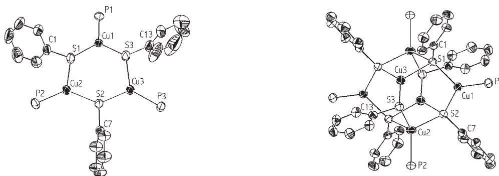
Figure 3. Molecular structures of [(^1\text{Pr}_3\text{PCuSPh})_3] (7) and [(^1\text{Pr}_3\text{P})_4(\text{CuSPh})_6] (8). Thermal ellipsoids are drawn at the 50% probability level. Hydrogen atoms and ^1\text{Pr} -groups are omitted.
